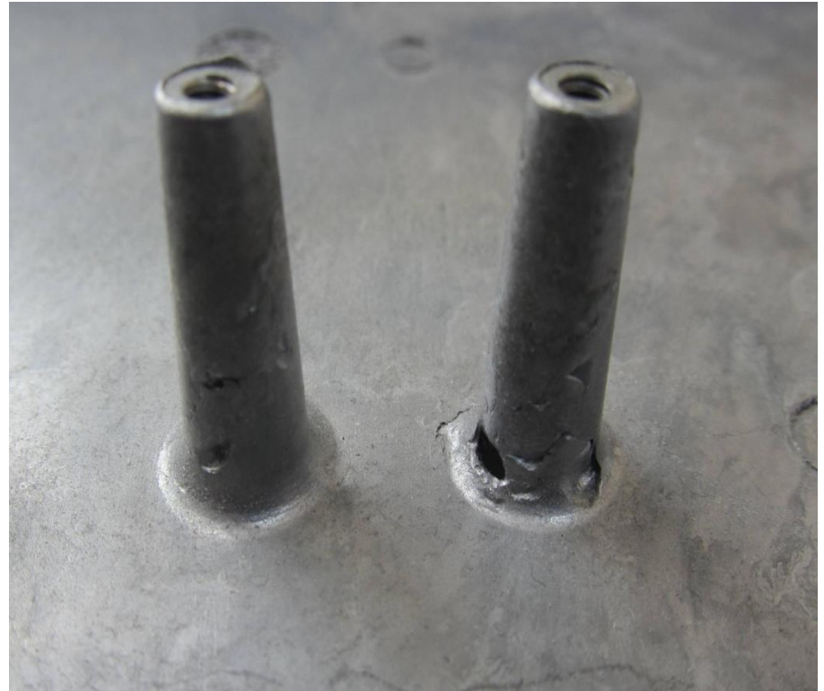
Porosity in an aluminum diecasting.
